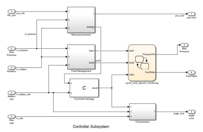
The Command Strategy block implements a look-up table using custom C code and outputs a value result based on two inputs x and y.
