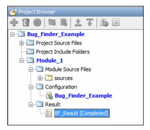
The Bug Finder (Code Prover) results are stored in a .psbf(.pscp) file in the results folder. For instance, if you save your project in C:\Projects\, a .psbf file for the Bug Finder analysis results on the first module Module\_1 is stored in C:\Projects\Module\_1\BF\_Result. See also "Project and Results Folder Contents" on page 1-11.
